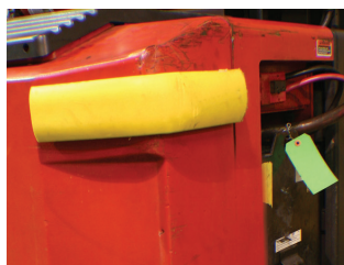
Using two way tape, non-metal surfaces can be protected
