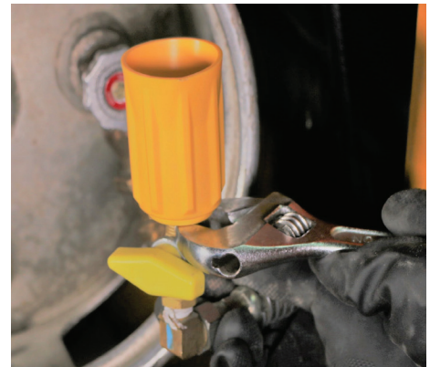
INSTALL COUPLER ON PROPANE VALVE WITH A WRENCH
